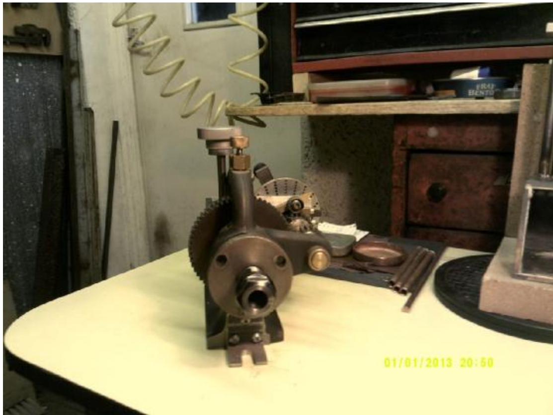
The spindle has a No.1 Morse taper and takes an ER20 collet chuck with a 6mm drawbar for small items. A bracket was made for holding down, the other is in the main casting.
