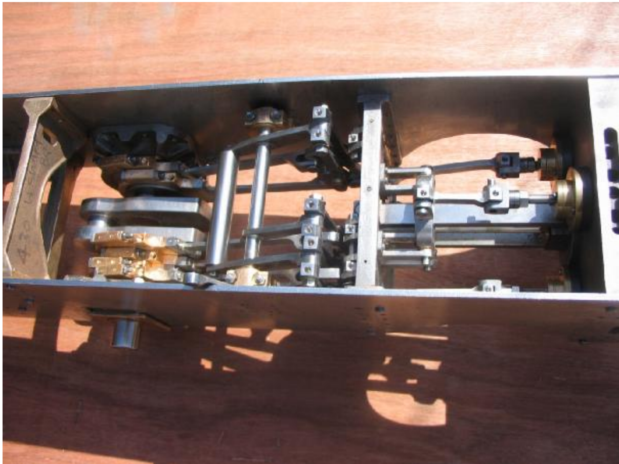
Top View of the Valve gear set-up (note the six lifting links)
